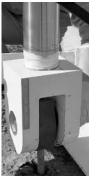
Using a transit, anchor creep is monitored as load is applied to the installed anchor.
