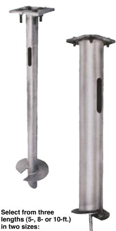
pecifically designed for above-grade and on-grade mounting of parking-area/site lighting standards, these non-extendable foundation anchors have high-strength pipe shafts to resist bending moments and substantial installing-torque ratings.
